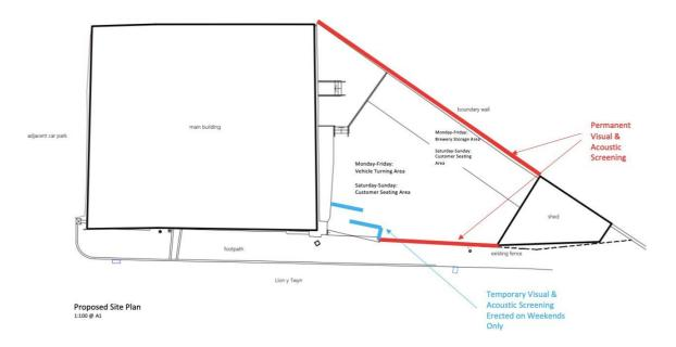
Note that both the main brewery building and the shed are heavily insulated concrete structures that require no further acoustic screening as they are already extremely effective at blocking any sound.
